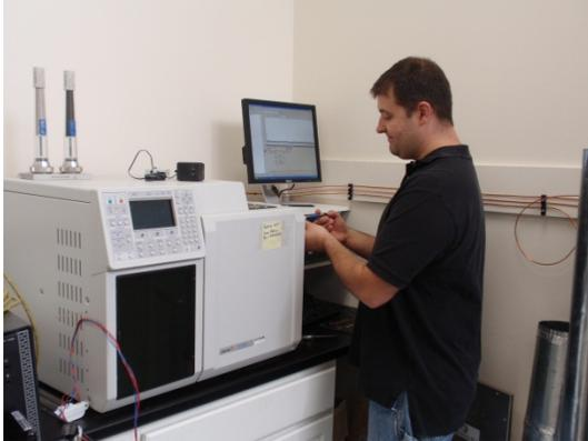
Gas Chromatograph to measure ethylene
